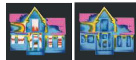
Before siding installation, energy transfers through the studs and siding.
